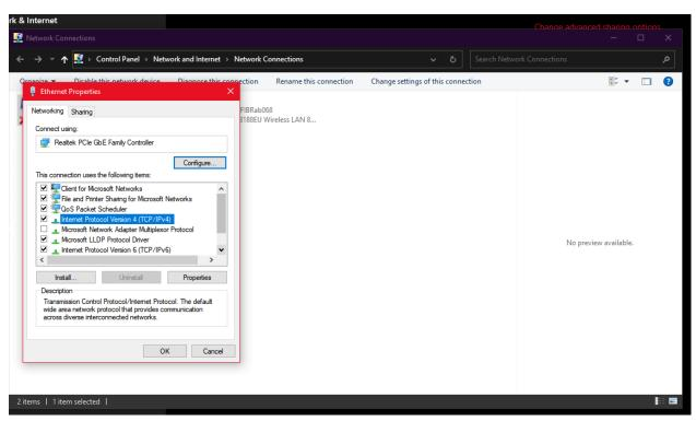
Step 6: Select "Use the following IP address and on the empty field, type in 192.168.1.101. The subnet mask will be automatically be filled out. Click OK and close all the open windows.
